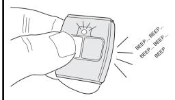
PROGRAM THE TRANSMITTER INTO THE RECEIVER BY PLACING THE RECEIVER INTO PROGRAM MODE, THEN SEND A SIGNAL TO THE RECEIVER FROM THE TRANSMITTER. REFER TO THE RECEIVER'S PROGRAMMING INSTRUCTIONS
